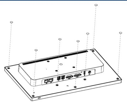
**Step 1.** Remove 7 Screw Mylar from the panel.
